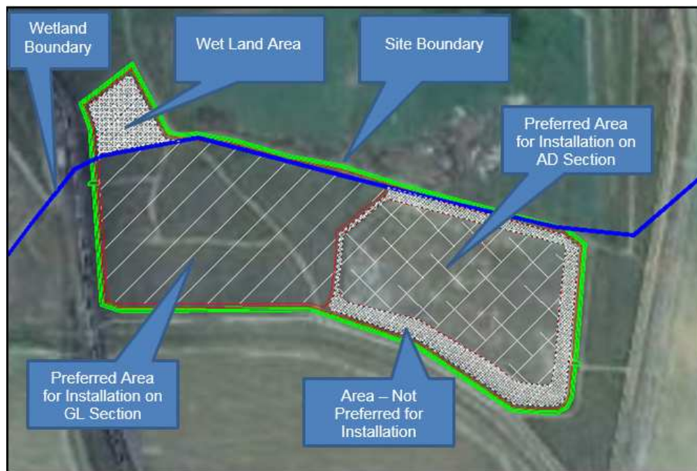
Figure 3-2: Area Suitable for PV Installation
